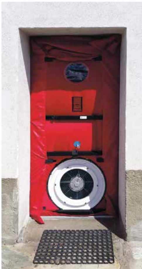
Figura 6.37: Test blower door.
